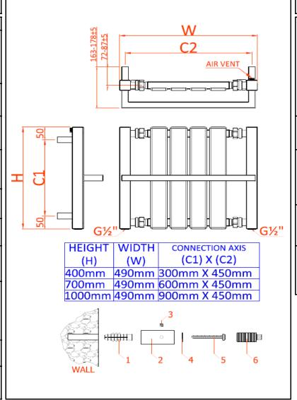
The radiator should not be mounted closer than 50mm below any overhanging surface (i.ei shelf) and no lower than 100mm from the floor. Transfer the bracket drill position measurements to the wall.
