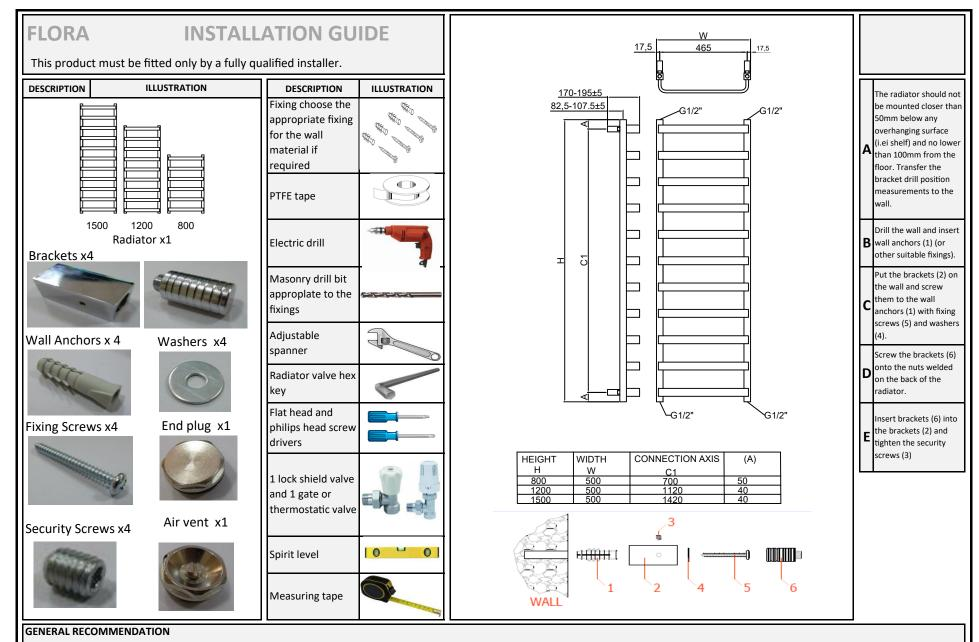
Before fitting the radiator it is necessary to wash out the heating system to remove any existing mud, scale, work residues, traces of flux, oil, etc.
