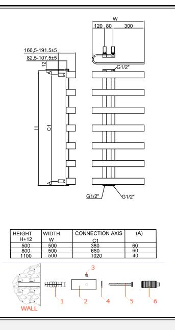
The radiator should not be mounted closer than 50mm below any overhanging surface (i.ei shelf) and no lower than 100mm from the floor. Transfer the bracket drill position measurements to the
